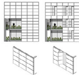
Shaders Structure | Opening system
